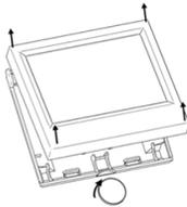
1 – Separate the thermostat from the base with a coin
