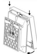
3 - Reassemble thermostat to its base as indicated in the picture.
